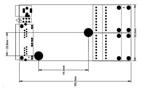
Positioning hole size inner diameter 3.5MM outer diameter 6MM
